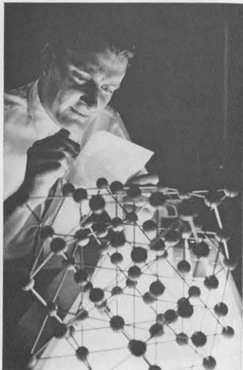
MOLECULAR MODELS such as the one in the foreground are prepared by Analytical Section II, 1122-2, using information derived from X-ray crystal studies. Ed Graeber of the Section examines radiograph of crystal, made with the Buerger Precession Camera.
